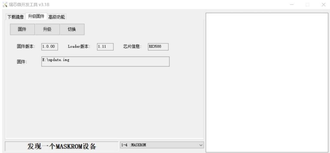
Click the "Firmware" button to load the firmware, and then click the "Upgrade" button.
